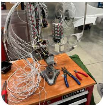
Wiring up the new panel for the avionics upgrade
